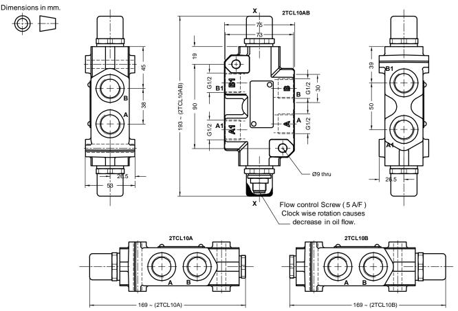
Note : Rotate the valve around horizontal axis 'X' - 'X' by 180° to convert from METER-IN control to METER-OUT control. Valve fixing S.H.C Screws are not in scope of supply. Tightening torque for M8x1.25 S.H.C Screws is 39 Nm.
