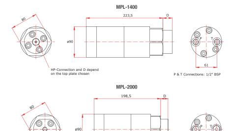
The HP-Connection and D depends on the top plate chosen.
