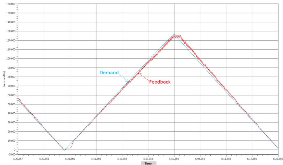
The accuracy of both applications can be trimmed by honing the pseudo PID control parameters, size of test piece (i.e. pressurised volume), degree of air entrapment and test piece expansive volume. This will all affect the accuracy however, simple programme parameters can be adjusted to meet the demand within the precision of the transducer.
