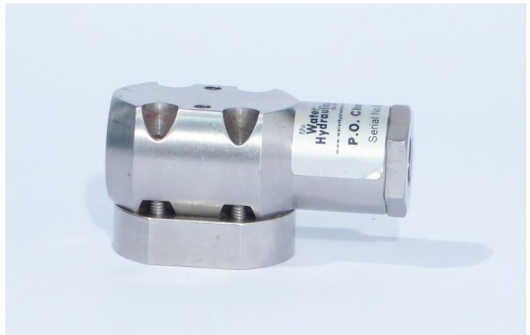
They are offered as either single or double port checked. The valve can be used for locking a water cylinder in a stationary position. Actuation can only occur when the required pilot pressure is available. A port adaptor block is also available for remote use, e.g. cylinder mounted.
